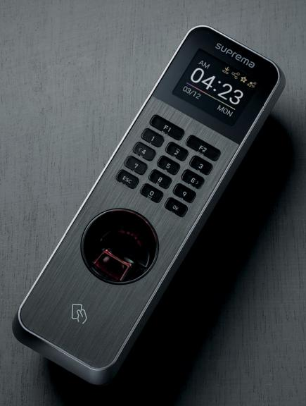
Suprema BioLite N2 is a Suprema's 2nd generation outdoor fingerprint terminal that provides comprehensive access control and time attendance features based on Suprema's latest biometric technology and security platform. BioLite N2 provides class-leading performance and security by featuring Suprema's latest fingerprint algorithm coupled with world's best fingerprint sensor. Packed in a rugged IP67 housing, BioLite N2 added flexibility in system design with multi-class RFID reading technology.
