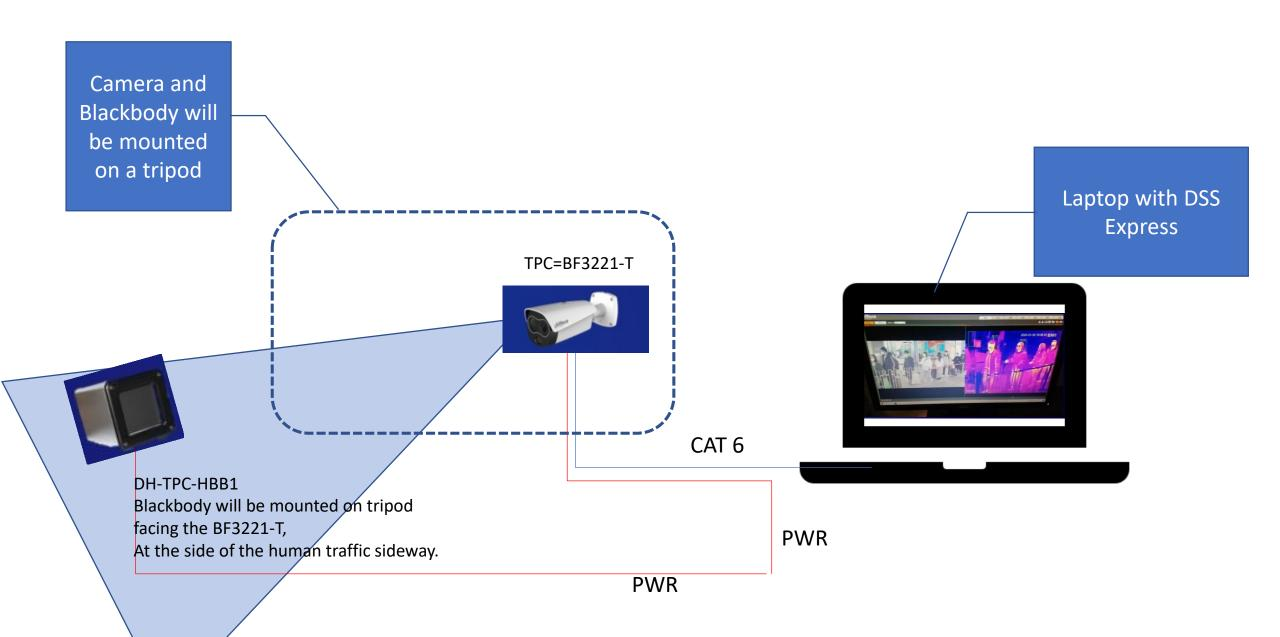
Deploy the thermal camera facing the human traffic direction,
