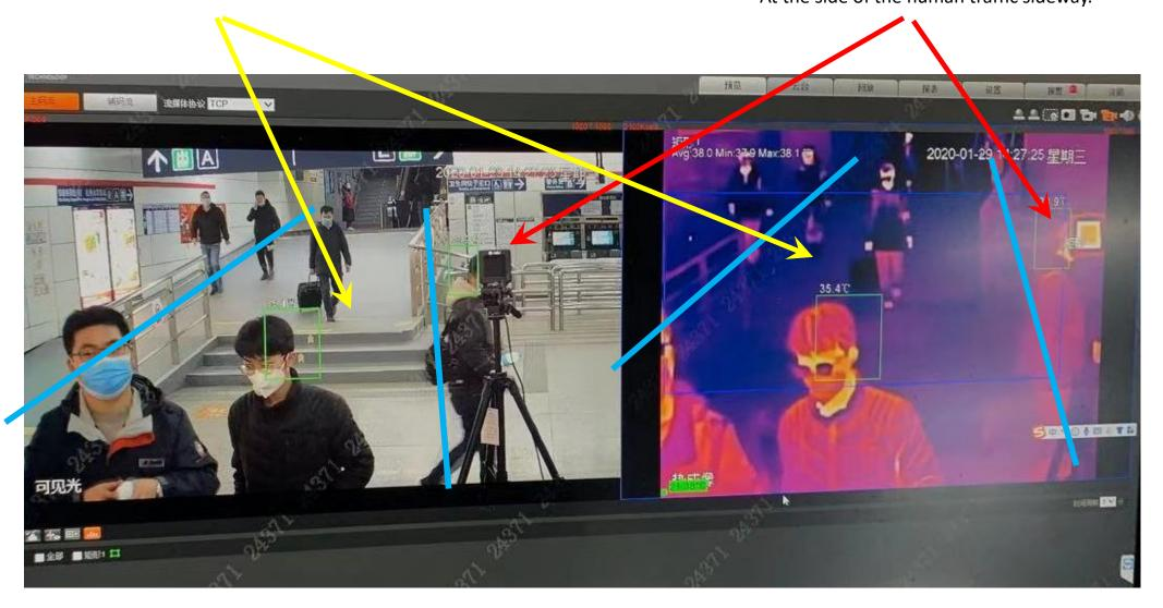
Deploy the thermal camera facing the human traffic direction,
